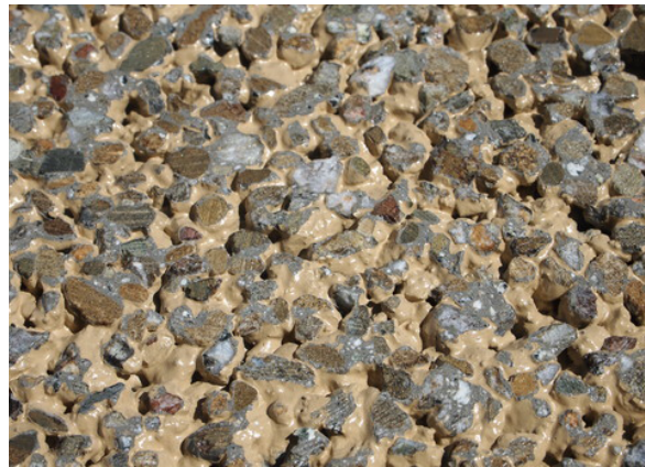
Larger aggregate size of pervious concrete pavement, with integral color
